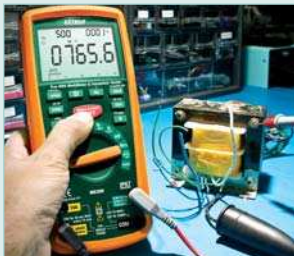
Measure the insulation resistance of transformer windings
