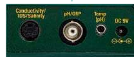
Side inputs for Conductivity Cell, pH/ORP probe, Thermistor probe, and AC Adaptor
