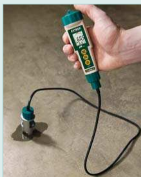
Extension cable and weight attached to meter and electrode module for easy measurement on concrete
