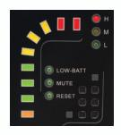
Extech's Refrigerant Leakage Detector is easy to use and is ideal for detecting leakages from air-conditioning units and cooling systems that use all standard refrigerants. The multi-colored LED light bar indicates the level of leaking refrigerant detected by the RD300. The built-in, bright LED convenience light located at the sensor tip illuminates dimly lit inspection areas.
