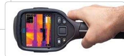
Auto-Orientation Keeps Diagnostics Overlays Upright
