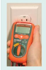
Built-in Non-Contact Voltage Detector. Red LED bar lights when live wire detected.
