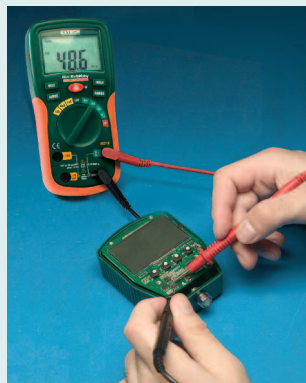
AC/DC Voltage measurements
