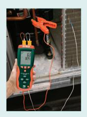
Take differential temperature readings with dual Type K thermocouple probes. Shown above with bead wire Type K thermocouple probe (included) and optional TP200 Type K Pipe Clamp Probe.
