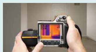
Infrared cameras quickly locate moisture related problems
