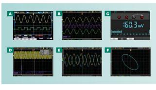
5.6" (142mm) graphical color LCD for viewing multiple waveforms plus built-in digital multimeter display and analog bargraph.
