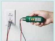
Take voltage measurements using the attachable test lead tip (RC200-TL)
