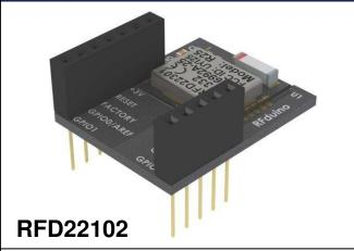
DIP version of RFD22301 for prototyping
