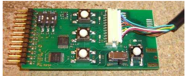
RFD21772 / RFD21773 Eval board with RFDANT cable plugged into the 11 pin connector.
