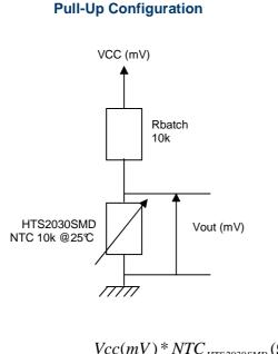
$$V_{OUT}(mV) = \frac{Vcc(mV) * NTC_{HTS 2030SMD}(\Omega)}{R_{batch}(\Omega) + NTC_{HTS 2030SMD}(\Omega)}$$
