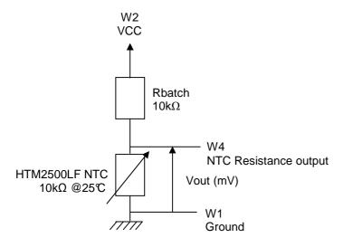
$$V_{OUT}(mV) = \frac{V_{CC}(mV) * NTC_{HTM 2500LF}(\Omega)}{R_{batch}(\Omega) + NTC_{HTM 2500LF}(\Omega)}$$
