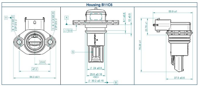
Recommended Screw Mounting: M6; Typical tightening torque: 12 N.m; Maximum tightening torque: 17 N.m
