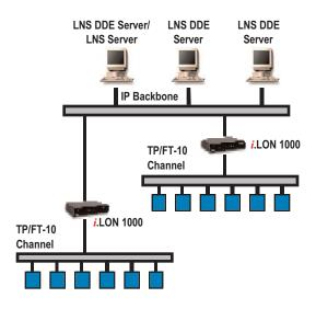
The LNS DDE Server can be used on a PC that is connected to an IP backbone, that is in turn connected to many channels via *i*.LON<sup>®</sup> 1000 Internet Servers. This provides the highest performance for monitoring and control applications. The *i*.LON 1000 Internet Servers aggregate traffic from their channels, providing efficient utilization of the IP backbone channel, and maximizing the number of packets per second that can be processed by the LNS DDE Server PC.
