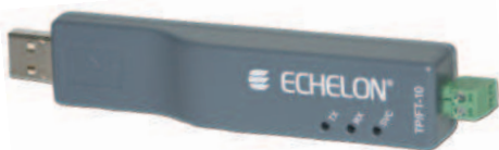
U10 USB Network Interface – TP/FT-10 Channel
