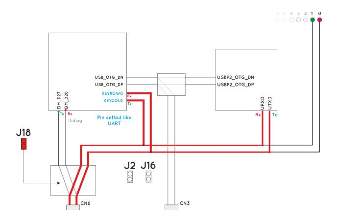
After the OS boot, the connection between the two processors is established and working. For this reason, it is impossible to connect an external Host PC through microUSB connector CN6 (without J18 jumper inserted), since it would result in the unusability of the shared serial port. The same situation occurs when trying to communicating with UDOO board through pins 0 and 1 of the Arduino Due – pinout compatible pin headers, since SAM3X8E UART Serial Rx and Tx line are wired also on these pins.
