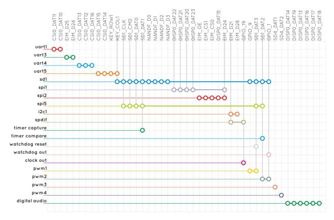
Looking at the previous diagram, on the vertical axis there is the functionality provided by iMx6. On the horizontal axis are shown the pins used to implements each functionality. Be careful that some pins are used for different functionalities and only one at a time can be active for each of them.
