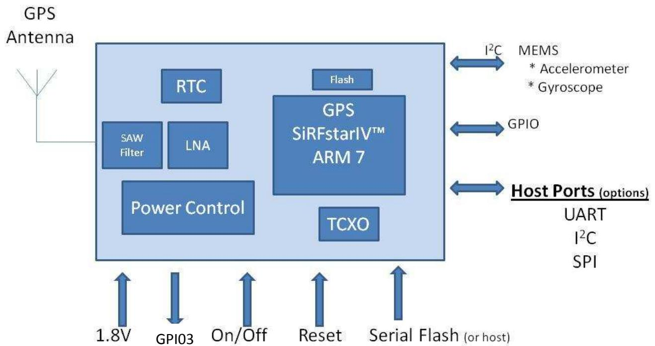
Figure 1 Inventek's ISM480F1 General Block Diagram
