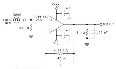
PULSE GENERATOR: 1. RISE TIME ≤ 10 ns 2. REPETITION RATE, 1 kHz(MAX)
