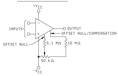
FIGURE 2. Offset null circuits.
