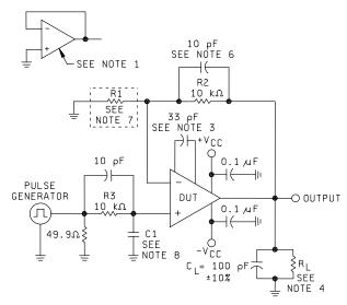
PULSE GENERATOR: 1. RISE TIME ≤ 100 ns 2. REPETITION RATE, 1 kHz(MAX)
