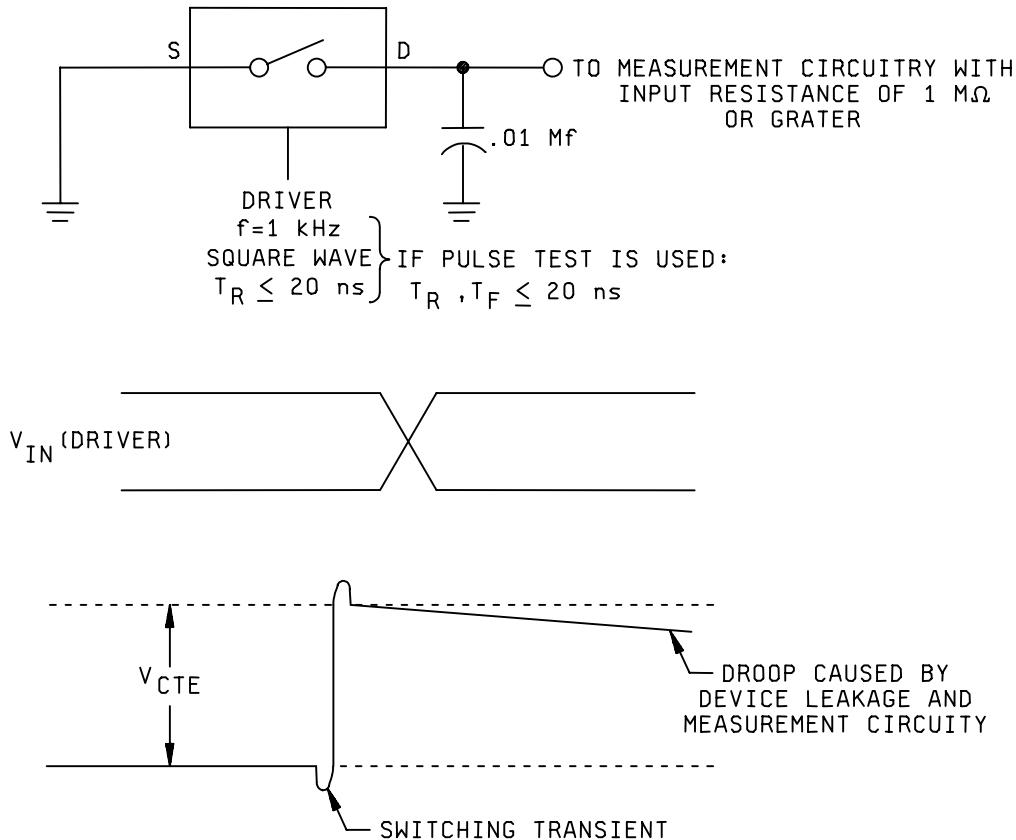
FIGURE 13. Charge transfer error test circuit.
