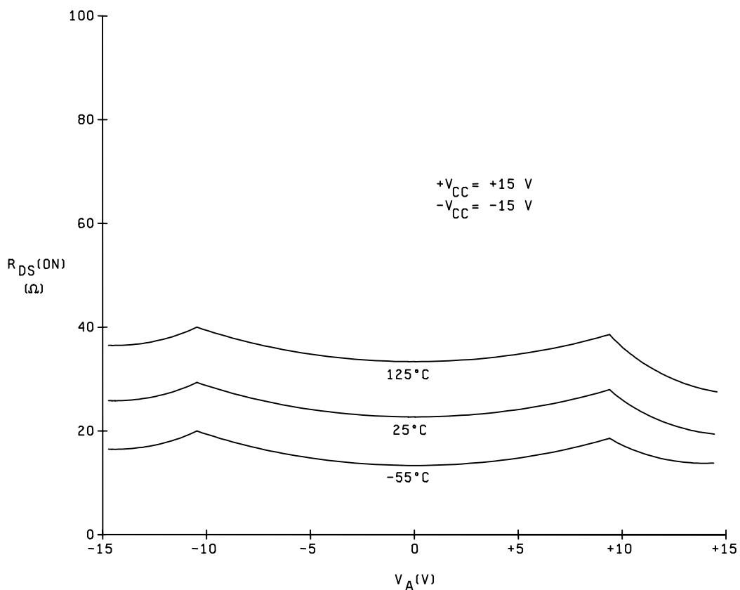
Figure 2.  $R_{DS(ON)}$  versus  $V_A$  and temperature.
