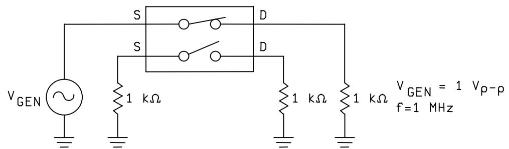
FIGURE 12. Crosstalk test circuit.
