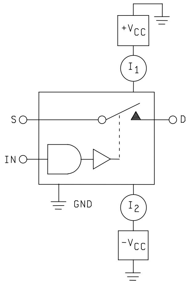
Figure 6.  $I^+$ ,  $I^-$  test circuit.
