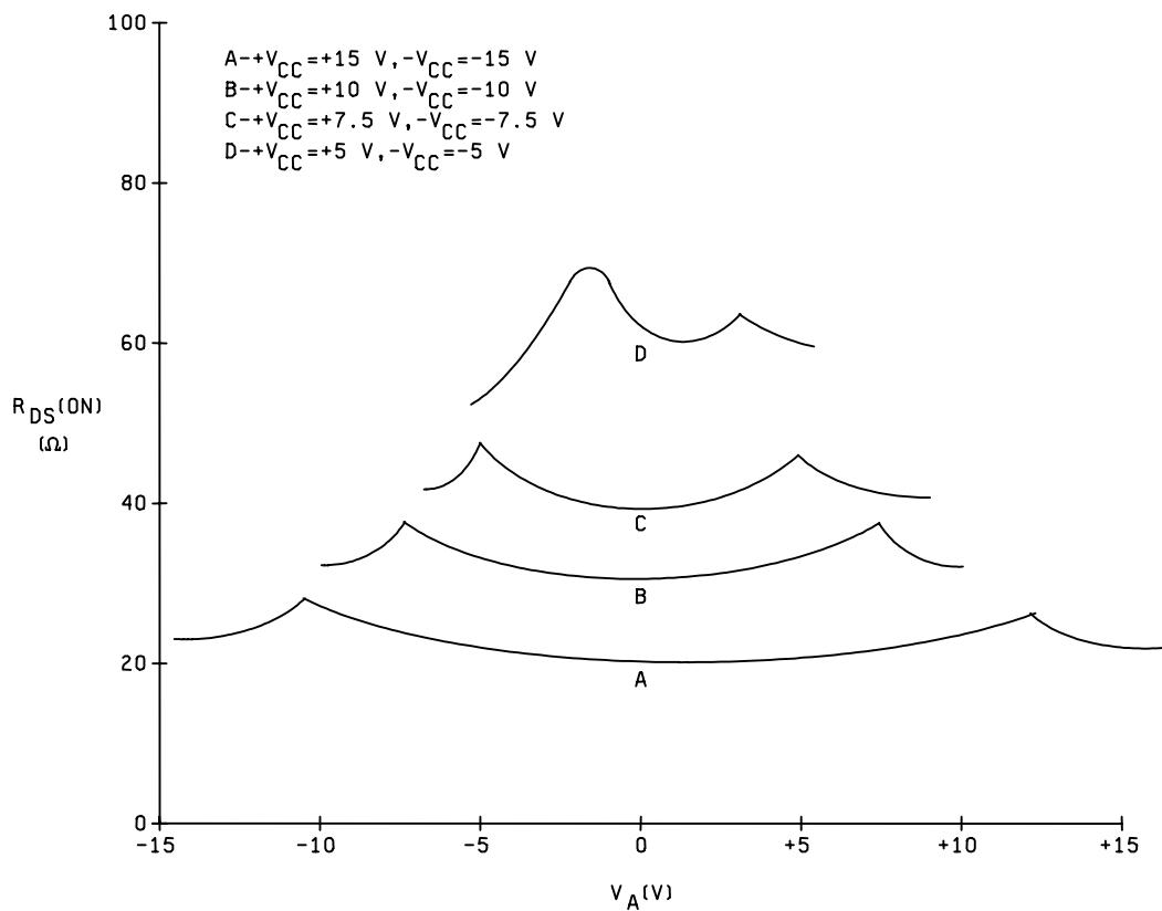
Figure 1.  $R_{DS(ON)}$  versus  $V_A$  and power supply voltage.
