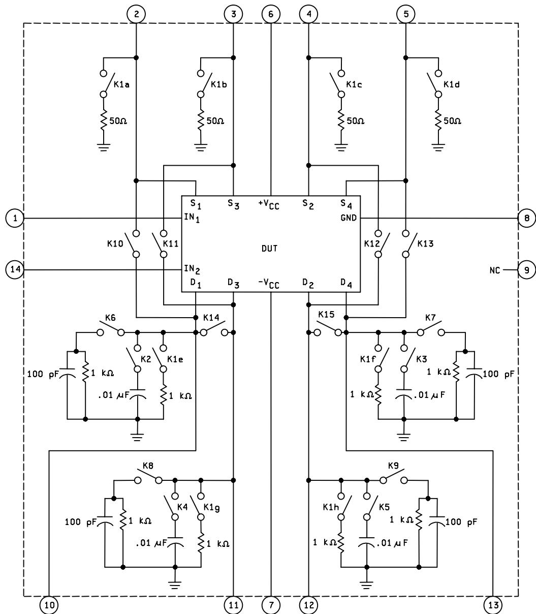
FIGURE 17. Test circuit (static and dynamic tests) for device types 03, 04, 07, and 08.
