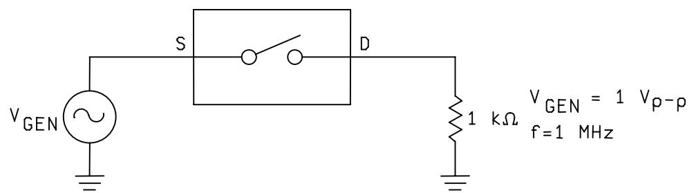
FIGURE 11. Isolation test circuit.
