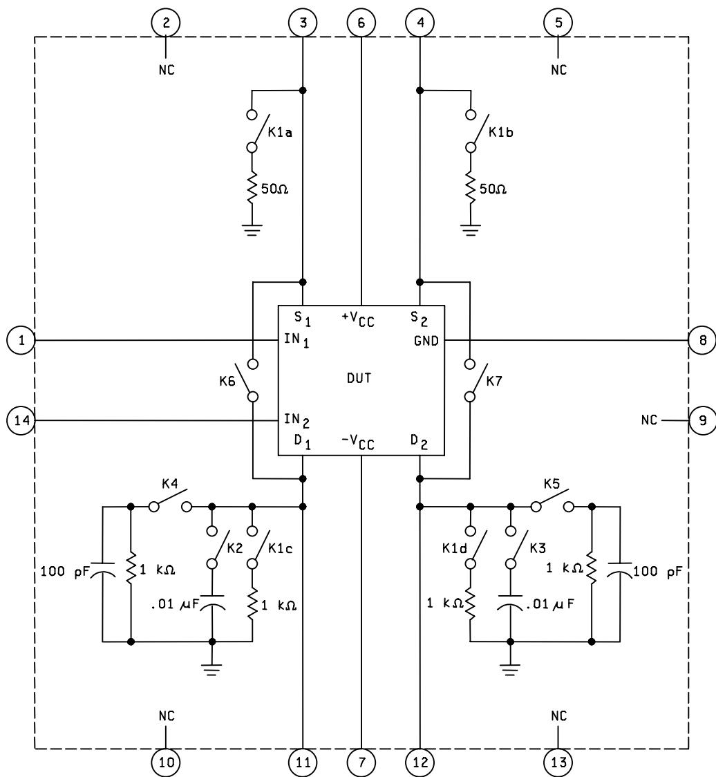
FIGURE 15. Test circuit (static and dynamic tests) for device types 01 and 05.
