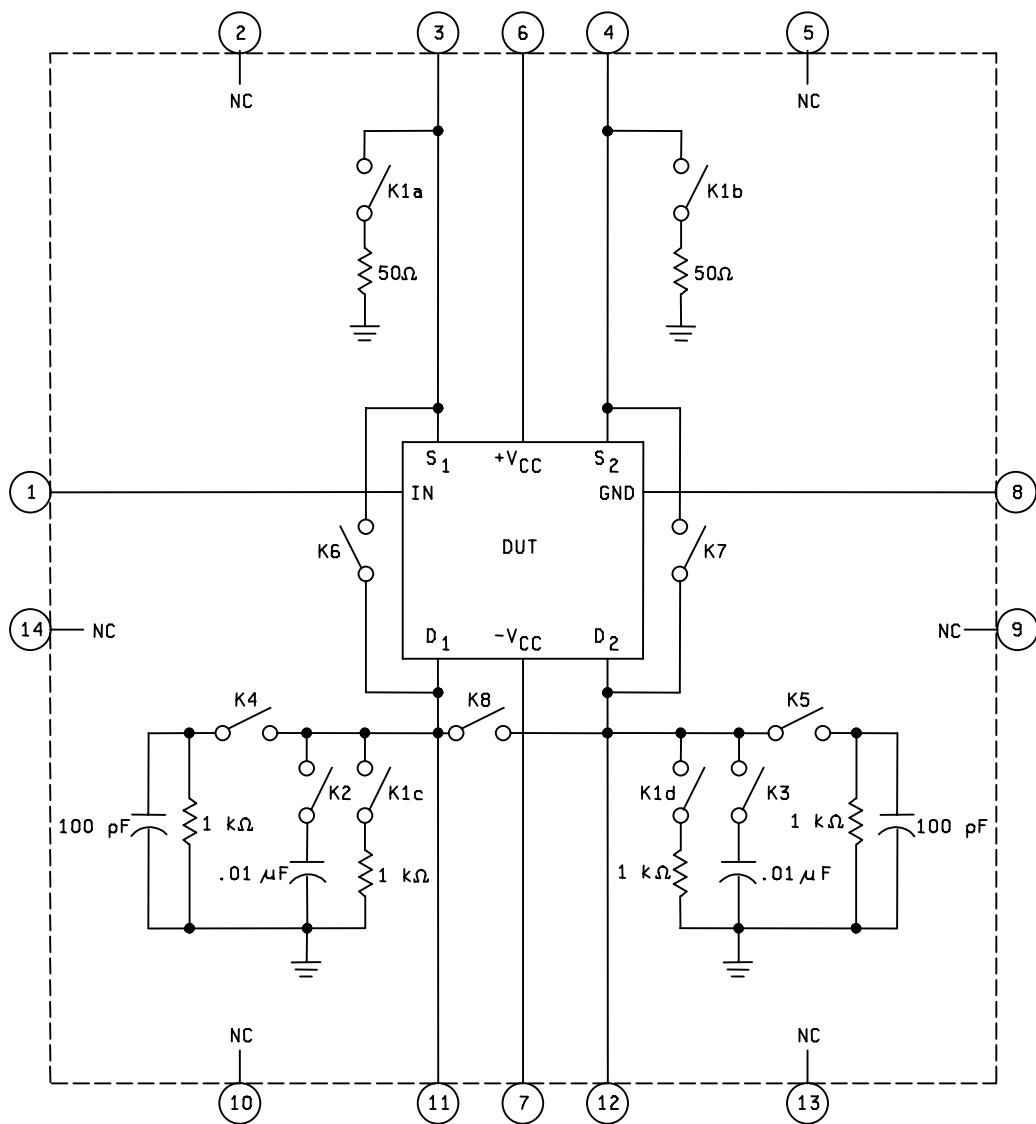
FIGURE 16. Test circuit (static and dynamic tests) for device types 02 and 06.
