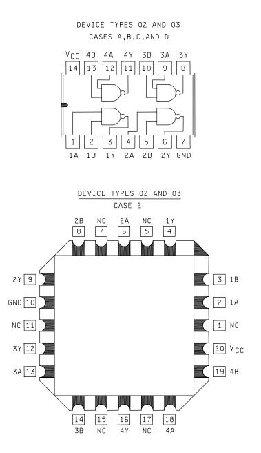
FIGURE 1. Logic diagram and terminal connections (top views) - Continued.
