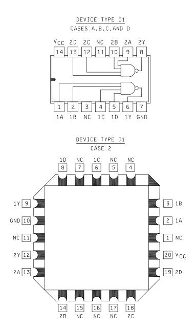
FIGURE 1. Logic diagram and terminal connections (top views).
