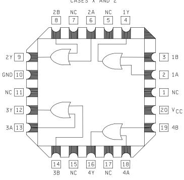
FIGURE 1. Terminal connections and truth table.
