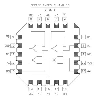
FIGURE 1. Terminal connections and logic diagram (top view).
