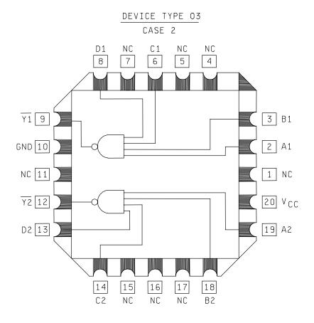
FIGURE 1. <u>Terminal connections and logic diagram</u> Continued.
