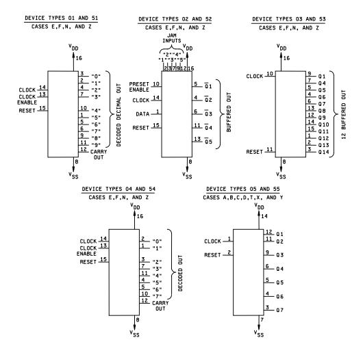
FIGURE 1. Terminal connections.
