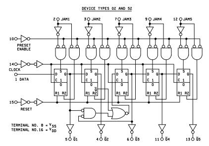
SHOWN IN "DIVIDE BY TEN CONFIGURATION," Q5 TIED DIRECTLY TO DATA INPUT.
