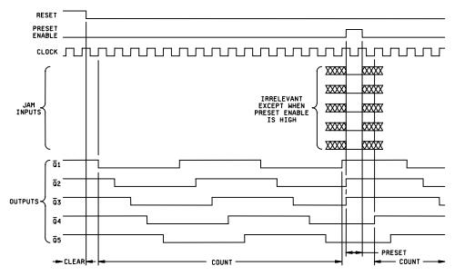
FIGURE 2. Logic diagrams and functional waveforms - Continued.
