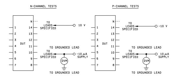
FIGURE 9. Threshold-voltage test circuit.
