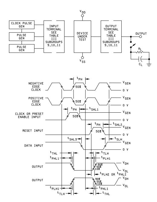
FIGURE 8. Switching time waveforms and test circuit.
