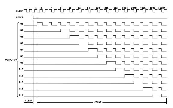
FIGURE 2. Logic diagrams and functional waveforms - Continued.
