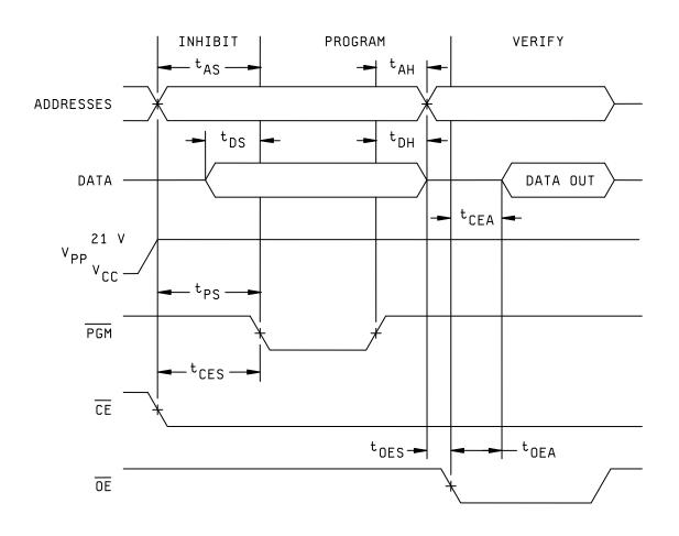
FIGURE 6. Programming timing diagram for method A.
