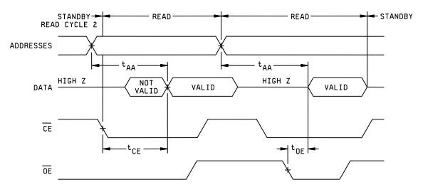
FIGURE 5. Read cycle timing diagram - Continued.
