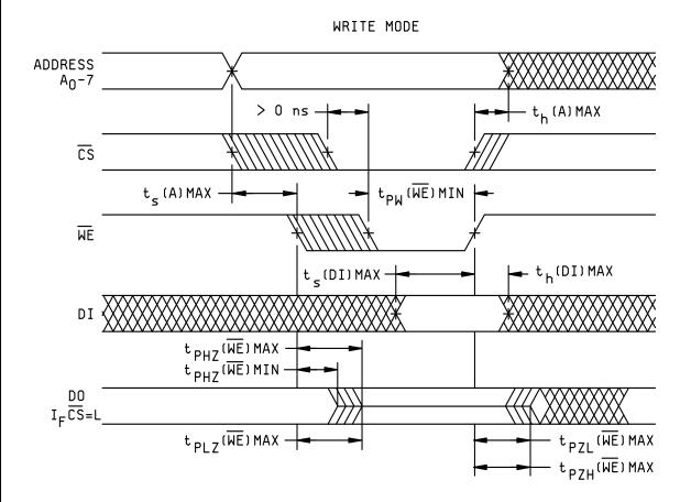
Write Cycle Timing. The cycle is initiated by an address change. After  $t_s(A)$  max, the write enable may begin. The chip select must also be LOW for writing. Following the write pulse,  $t_h(A)$  max must be allowed before the address may be changed again. The output will be inactive (floating for device types 01 and 02) while the write enable is LOW. Ordinarily, the chip select should be LOW during the entire write pulse.
