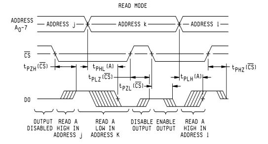
Switching delays from address and chip select inputs to the data output. For devices 01 and 02, disabled output is "OFF", represented by a single center line. For devices 03 and 04 a disabled output is HIGH.
