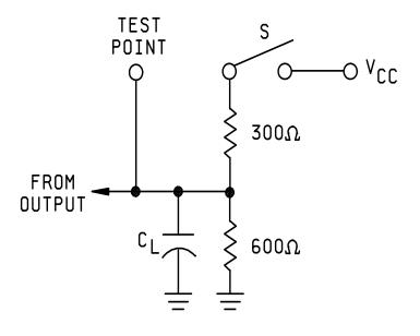
FIGURE 4. Switching test circuit.
