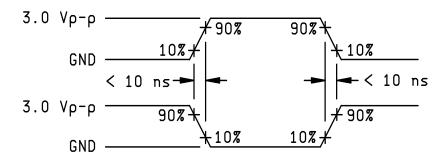
FIGURE 5. Switching test waveform.
