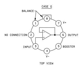
FIGURE 1. <u>Terminal connections</u> - Continued. (Internal)
