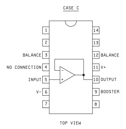
FIGURE 1. Terminal connections. (Internal)
