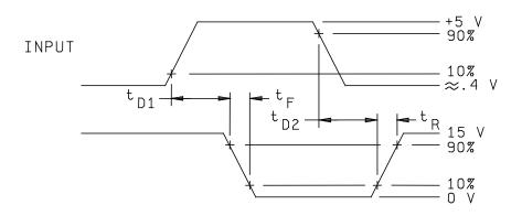
FIGURE 2. Timing waveforms.
