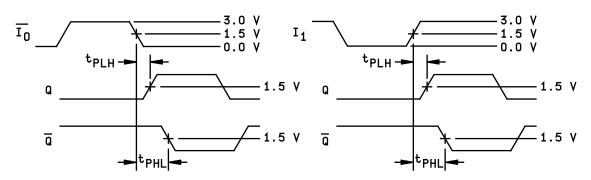
FIGURE 4. Switching waveforms and test circuit.
