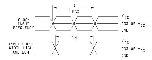
FIGURE 4. Switching waveforms and test circuit.
