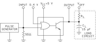
NOTE: C<sub>L</sub> includes probe and test fixture capacitance.
