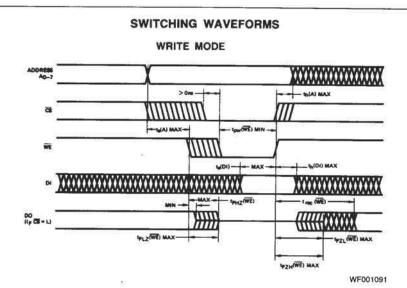
Write Cycle Timing. The cycle is initiated by an address change. After  $t_s(A)$  max, the write enable may begin. The chip select must also be LOW for writing. Following the write pulse,  $t_h(A)$  max must be allowed before the address may be changed again. The output will be inactive (floating for the Am27LS00A/00) while the write enable is LOW. Ordinarily, the chip select should be LOW during the entire write pulse.
