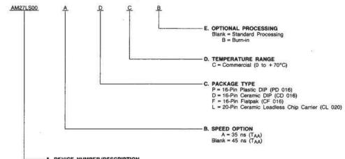
DEVICE NUMBER/DESCRIPTION Am27LS00/27LS00-1 Series Three-State Bipolar RAMs Am27LS01/27LS01-1 Series Open-Collector Bipolar RAMs
