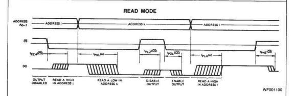
Switching delays from address and chip select inputs to the data output. For the Am27LS00A/00, Am27LS00-1A/00-1 disabled output is "OFF," represented by a single center line. For the Am27LS01A/01, Am27LS01-1A/01-1, a disabled output is HIGH.
