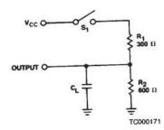
Notes: 1. TAVQV is tested with switch S<sub>1</sub> closed and C<sub>L</sub> = 50 pF. TEVAV is defined as chip enable setup time.
