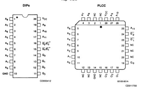
Note: Pin 1 is marked for orientation.
