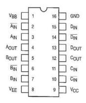
Pin assignment is for Dual-in-Line Package. For PLCC pin assignment, see the Pin Conversion Tables on page 6-11. 3
