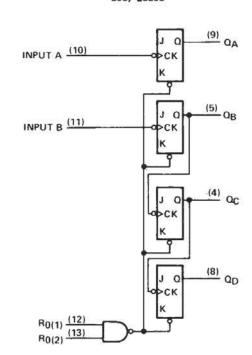
Pin numbers shown are for D, J, N, and W packages. The J and K inputs shown without connection are for reference only and are functionally at a high level.
