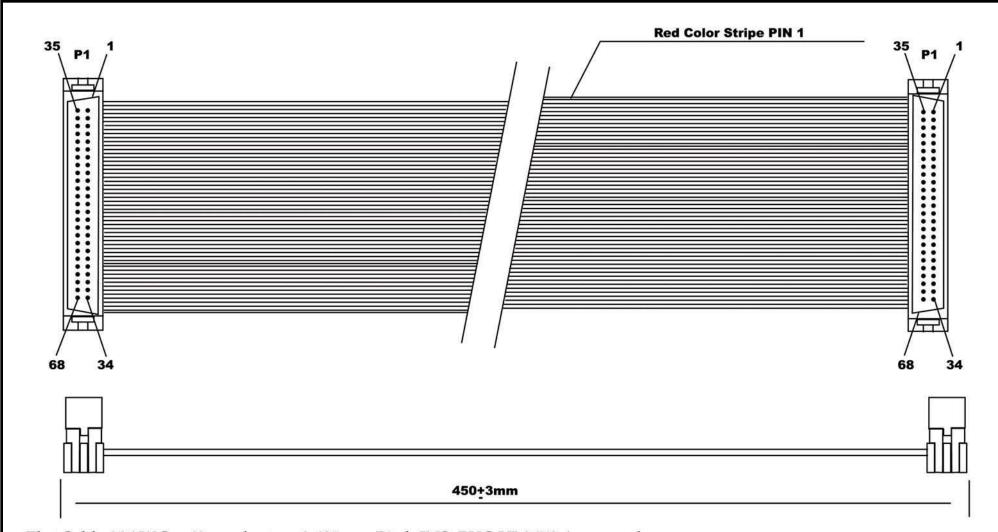
Flat Cable:28AWG x 68 conductors 0.635mm Pitch INS: PVC UL2678 Approved P1 IDC Plug 68PIN 1.27mm Pitch W/O Strain Relief Gold Flash Color:Black
