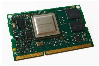
Maya is a ready-to-use CPU module based on Texas Instruments Cortex-A8 high performance application processor from DM814x (DaVinci) and AM387x (Sitara) families.
