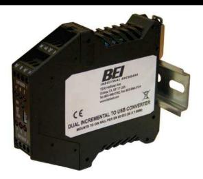
The Dual Encoder to USB Converter translates encoder position to industry standard USB 2.0 format that can be read by a computer. Each module can handle signals from two encoders. Modules are available for SSI absolute encoders, as well as quadrature incremental encoders.
