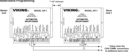
\* Note: The CAN COMM. terminals are polarity sensitive. \*\* Note: To avoid audio ring coupling, space units at least 3.0" apart.
