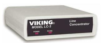
The LC-3 Line Concentrator allows up to three emergency phones to share a single line. A call initiated by any emergency phone is given the line. If a second emergency phone attempts to make a call while another emergency call is in use, the LC-3 will provide a busy signal until the line is available. Viking emergency phones can be programmed to redial on busy.
