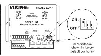
Note: Place DIP switches in the desired position then momentarily power down the unit.
