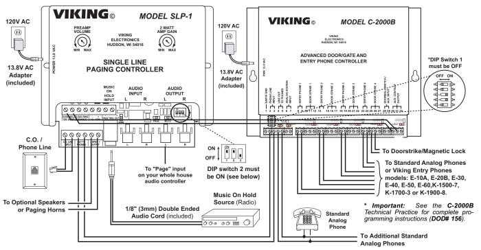
Important: With a C-2000B as the controller, the rev level of the SLP-1 must be REV F or higher in order for this application to work. If the controller is a C-2000A, the rev level of the SLP-1 must be no higher than REV E.
