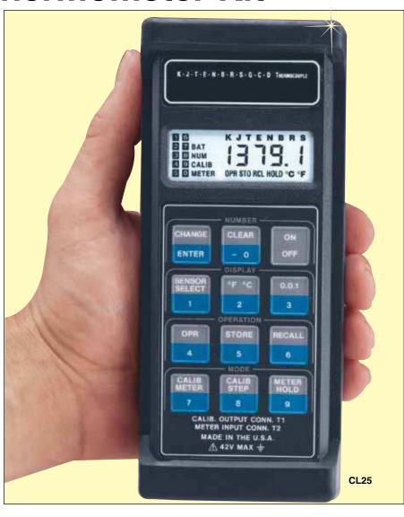
Simulates, Measures, and Records Thermocouple, RTD, Thermistor, and Resistance Signals—All in One Meter!
