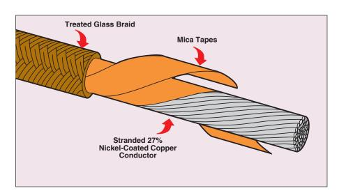
HTMG high-temperature lead wires are designed for appliances and industrial heating products—such as commercial food service equipment, heaters, heat treating furnaces, kilns, heater elements and other applications up to 450°C (842°F).
