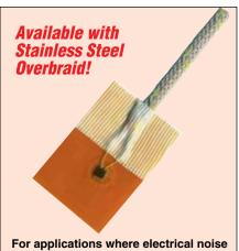
is prevalent, or where the sensor lead wires may be routed around sharp objects, consider the stainless steel overbraid option. To specify this option, add "-SB" to the end of the model number for an additional cost per meter (foot). Ordering example: SA1-RTD-80-SB.
