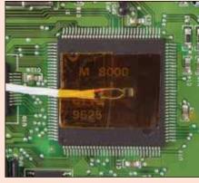
The self-adhesive sensor is ideal for "targeted" placement on curved or flat surfaces. Once in place, it can be used "as is" for measuring temperatures in applications such as machine tools, electronic products, structures or other places where temperatures need to be monitored and controlled.
