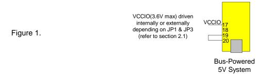
The figure above illustrates a typical USB bus-powered configuration. A USB bus-powered device gets its power from the USB bus.
