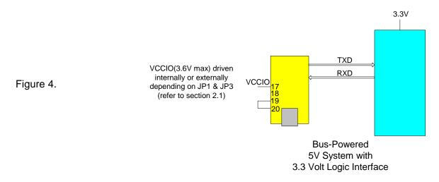
Figure 4 shows how to configure the DLP-2232H to interface with a 3.3V logic device via the ASYNC serial mode. In this example, the target electronics provide the 3.3 volts to power the microcontroller.
