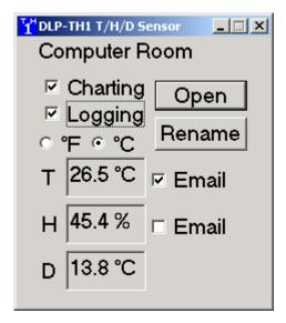
Since multiple DLP-TH1 units can be connected to the PC at the same time, when the program is run, the first required step is to select the sensor that is to be monitored. When the Open button is clicked, a selection window will appear that presents a list of all sensors connected to the PC. To select a specific sensor, simply click on the description string for the desired sensor and then click on OK.
