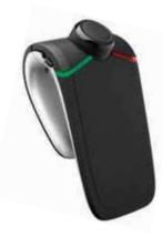
**Control the MINIKIT Neo by voice**: make and receive calls without touching any buttons. Say the key word 'MINIKIT' at any time to trigger the voice recognition, and then say the name of the contact you wish to call. When receiving a call, just say 'Accept' or 'Reject'. The kit recognises any voice without need for any programming, matching or training.
