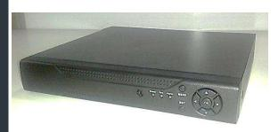
Streaming Scenarios Stream Case 1 Case 2 Encode **Primary** 30fps/ch 30fps/ch Steam H.264 H.264 Encode Secondary 30fps/ch 30fps/ch Stream H.264 H.264 Encode 4 x G.711 Audio mono 16KHz mono 16KHz Stream Decode Audio mono16KHz mono16KHz Stream
